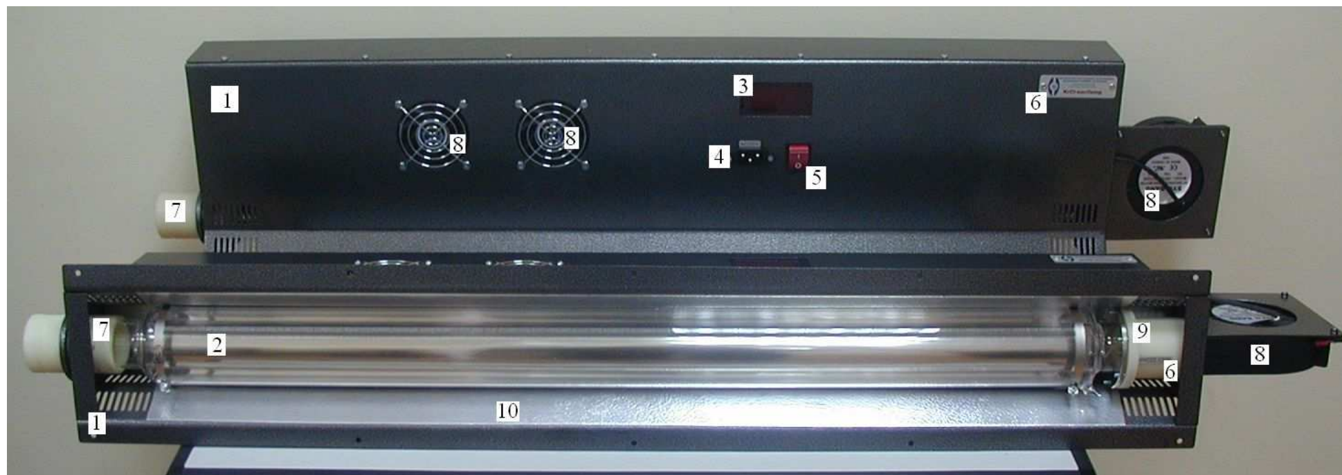
BD_EL excilamp photo: 1 – box; 2 – radiator; 3 – digital timer; 4 – AC network connector; 5 – AC network switch; 6 – nameplate; 7 – holder of radiator; 8 – fans; 9 – insulator of radiator; 10 – UV reflector
