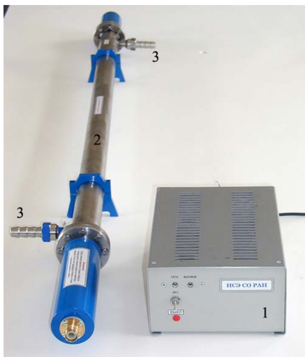
General view of BD_E_R photoreactor: 1 – power supply; 2 – reactor; 3 – connections for feed/outlet of the gas or solution.
